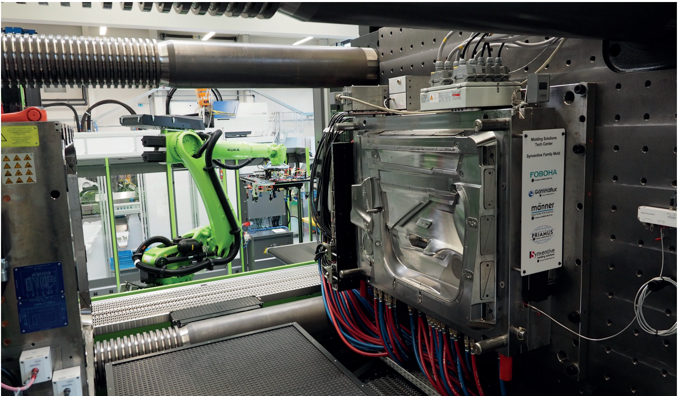
View into the mold space of the Engel Duo 2700 at the Tech Center. In the background, a 6-axis robot with 180 kg load-bearing capacity which removes the components. © Schröder/Hanser
