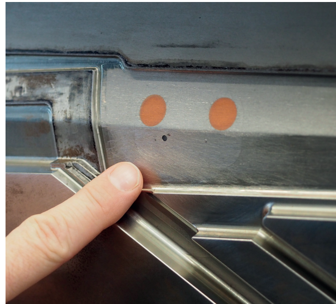
Fig. 4. Making a clear difference: one of 19 sensors installed in the mold. © Hanser/Schröder
